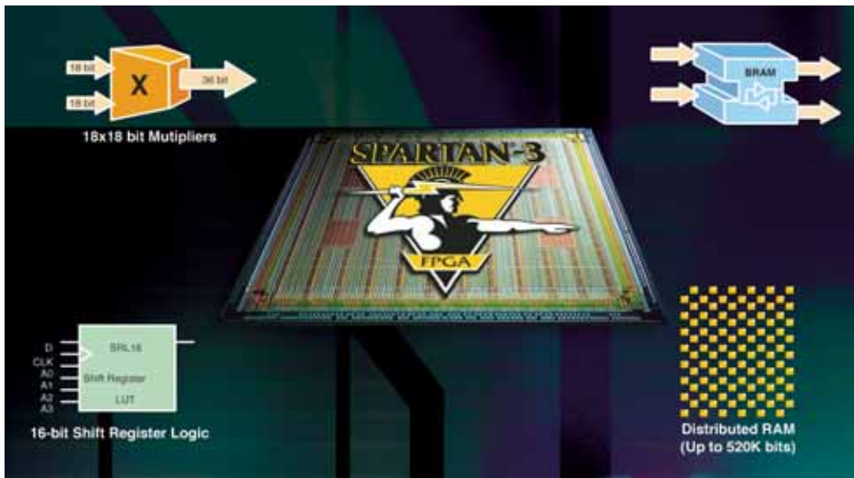
Figure 1 – Spartan-3 architecture optimized for lower DSP costs
