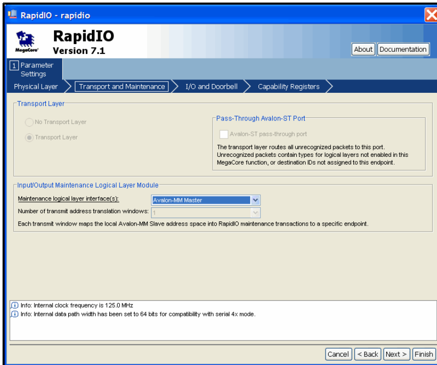
Figure 2–18. Transport Layer &amp; Maintenance Parameters
