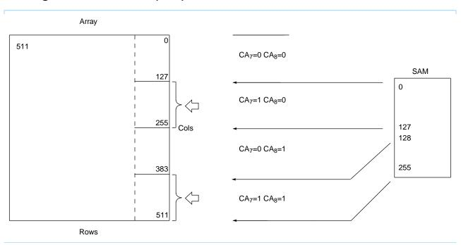
The example illustrates a full transfer in SRS mode based on CA<sub>7</sub>=1.
