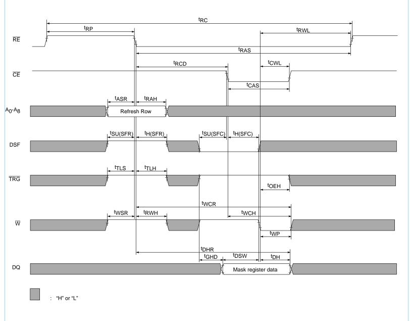
twcs tWCH tWSR <sup>t</sup>RWH  $\overline{\mathsf{W}}$ <sup>t</sup>DSC <sup>t</sup>DH Column mask for block "a" Column mask for block "b" DQ No mask (non-persistent or persistent) applied to BLOCK WRITE cycles.
