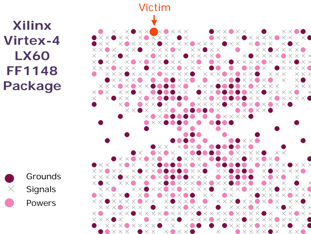
Figure 6—The LX60 package includes a well-distributed array of power and ground balls to control crosstalk.
